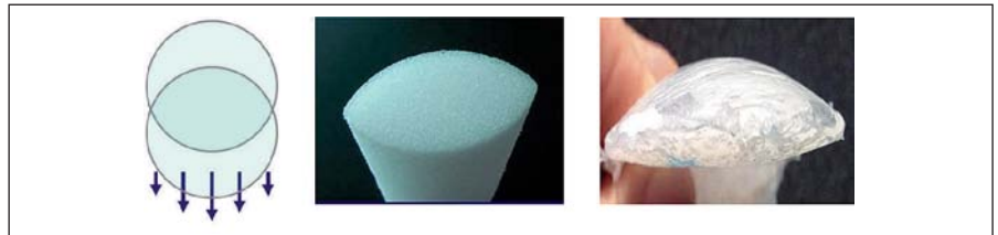
Fig. 1 a. Physical features of a compression device for a focally centred pressure, b. First implementation with foam. Aim: atraumatic borders and very stable positioning after contact pressure through concentric compression. c. Cross-section through an individual silicone compression device.
